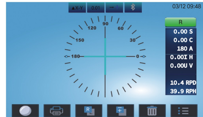
Figure 6.4 ADD display under measuring interface
