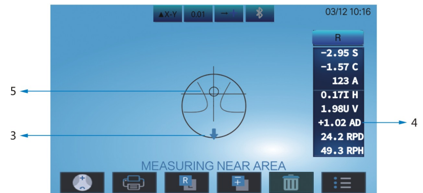
Figure 5.3 progressive lens measurement interface
